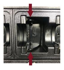
2. Pinch the railing to release it from the charger.
