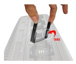
4. Snap the railing back into place. You may need to push it firmly until it fully locks.
